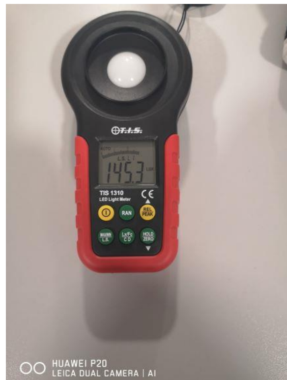
Fig 2 – Lux recording at table height ground floor kitchen of HPT is 145.3 Lumens
