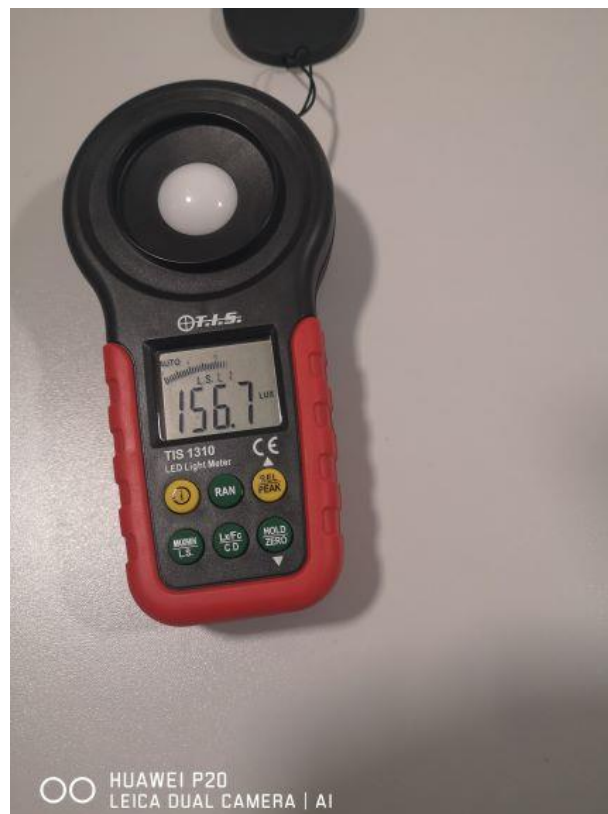
Fig. 4 showing the recorded level in the TV area 14 th floor, lux level 156.7 Lumens
